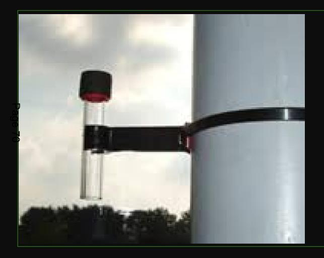
NO<sub>2</sub> Measured using Diffusion Tubes
